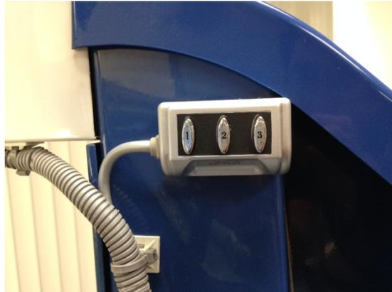
Figure 3: Remote control for camera selection
