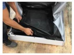
2. Replace the bag-retaining bars on the frame. The side bars must be placed slot-first under the adjacent front bar. Tighten the front bar fastener.
