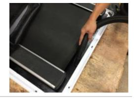
10. You can also check the surface of the treadbelt for debris or liquid spills. The treadbelt moves freely as you roll it by hand.
