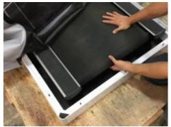
1. Reattach the bag, lining up the holes with the corresponding standoffs on the frame.
