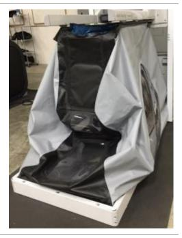
3. Locate the bag-retaining bars on the frame. The bars on the sides and rear are shown. You will remove these three bars. It may be easiest to start with the rear bar.
