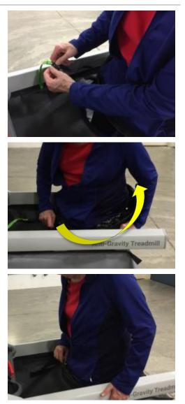
Always use the magnetic safety lanyard supplied with the Anti-Gravity Treadmill. If you lose the safety magnet, order a replacement from AlterG. As a precaution, the treadmill will not operate without the safety magnet directly over the Emergency Stop label.
