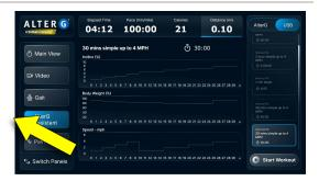
Select the source of the programmed workout by tapping either **AlterG** or **USB** on the upper right.
