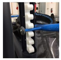
8. Close the safety latches located on the 2 front height adjusters. Press the latches down all the way and secure them with the spring-loaded safety pins.
