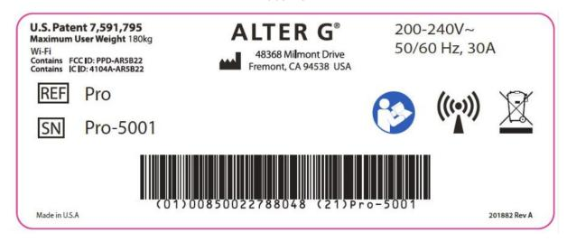
AlterG manufactures the system. This label is located on the base of the Anti-Gravity Treadmill and identifies the serial and model number of the system as well as the power and voltage requirements.
