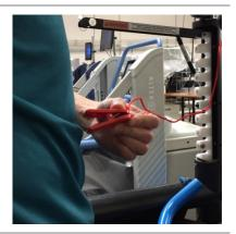
Place the lanyard safety magnet directly over the circular stud on the console labeled "Emergency Stop"; otherwise, the Anti-Gravity Treadmill will not operate.
