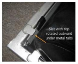
3. Slide the black plastic sliders under each metal tab on each side of the enclosure that you are reattaching.
