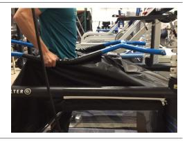
3. Use the numbers on the height adjusters as a reference and to ensure alignment between front, back and sides of the support frame. It is particularly important that the frame be level side-to-side.
