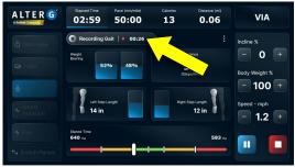
To activate cross-over gait mode, tap the Options menu to the right of the Record Gait button, and then select Cross Over Gait.
